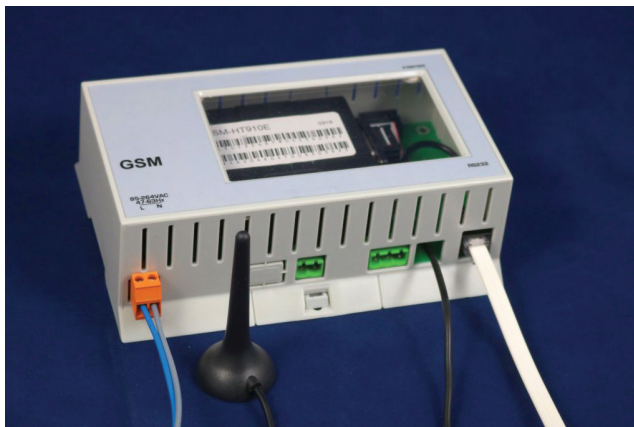
GSM controller module with RS-232 I/F to MiroWEB
